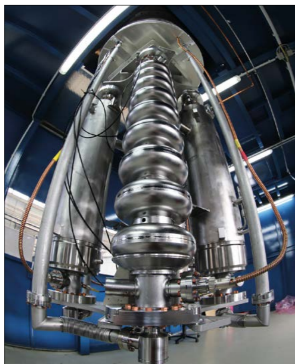
A superconducting cavity resonator for the European XFEL linac, measuring around 1 m long and pictured in a test configuration.
