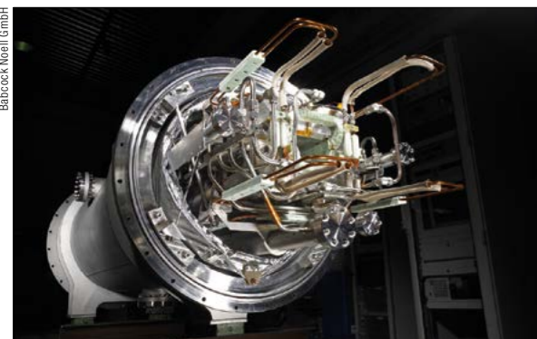
The newly developed fast-cycling superconducting dipole magnet for FAIR's SIS100 synchrotron.
