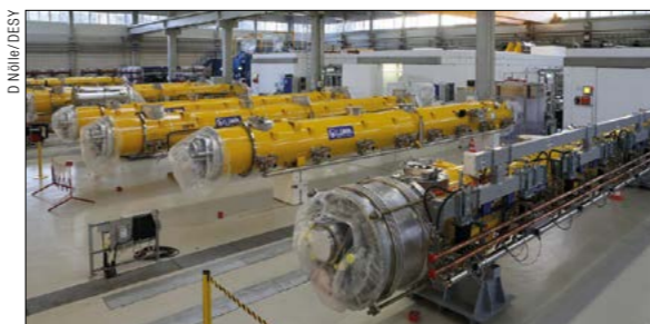
(Top) Connecting modules in the European XFEL linear accelerator. (Above) Superconducting accelerator modules in a test facility at DESY in October 2014.
